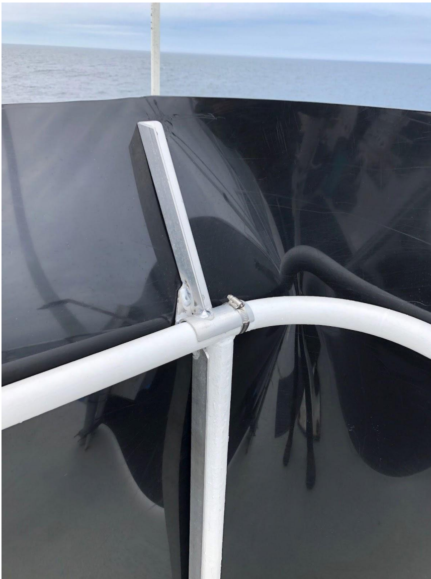
Close-up of temporary bracket holding top portion of windscreen, angled out to prevent wind directly over the top of screen. R/V Connecticut.
