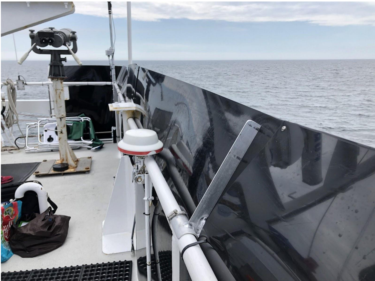
Big eye binocular stand, mounted to deck. Big eye binoculars mounted to stand. windscreen. R/V Connecticut.
